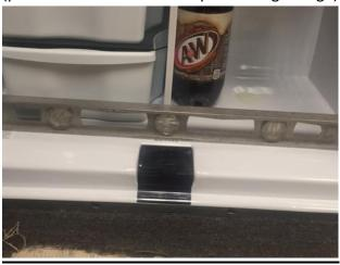
Paper Clip Test -Place paper clips all along the doors seal and the cabinet, as pictured below, to ensure no magnets have shifted in the cabinet. (paper clips need to be on both the seal and the
