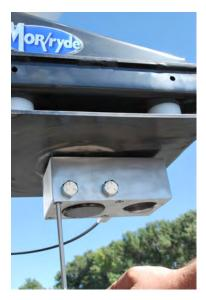
2-4. Using a 1/4" allen wrench, tighten the 4 set screws to about 40 ft-lbs of torque.
