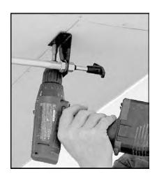
**IMPORTANT** The remote latch bracket should be installed within 30" of the center line of the ball socket to prevent the cable and bracket from being crushed by the pickup's sideboards. This can happen when the trailer and the pickup become twisted in reference to each other on uneven surfaces often found in campgrounds.
