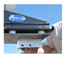
**2-1**. Place the kingpin coupler block on the kingpin as illustrated in the pictures to the left. Make sure the ball socket is face-down. For most 5th wheel installations, place the greaseless opening towards the front of the kingpin.
