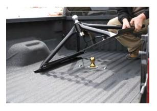
4-1. Place the Ultimate Connection in the bed of your truck so that the Ultimate Adjustable Ball is closest to the tailgate (as shown left).
