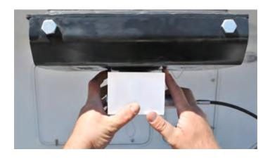
**2-3**. Make sure the coupler block is centered to the pin box before tightening the 4 set screws.
