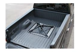
**4-2.** Place the pin through the lower coupler sleeve under the gooseneck ball and secure it in place with the hairpin clip. Push the entire base forward towards the cab of the truck until it will not go any further.
