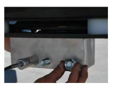
**2-2**. Insert the two 5" x 5/8" kingpin bolts into their holes to hold the coupler block on the kingpin and place the nuts on the two bolts as illustrated on the left. Push the bolts all the way flush to the block, but DO NOT fully tighten the nuts yet.
