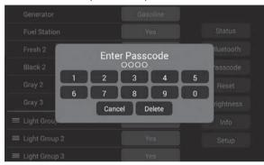
3. The passcode setup window will open. (Passcode protection may be disabled by selecting Change Passcode then Disable).
