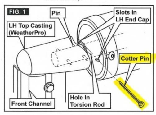
Insert 7/64" X 2-3/4" cotter pin (provided) through end cap and torsion rod. Then tape head of cotter pin to end cap to secure in place.
