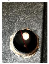
This is where you will insert the  $\frac{1}{4}$  "hex head bit and use cordless drill to rotate pump CW or CCW to extend or retract slides and hyd leveling legs
